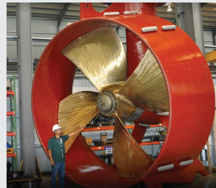
Workers inspect a marine thruster at the Houston manufacturing facility of Thrustmaster of Texas.
